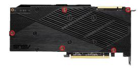
Remove cooler - 7x screws
