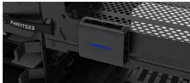
PWM hub upgrade (PH-PWHUB_01)
