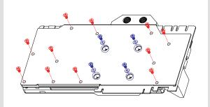
Use the included 4x M2.5x5 screws and washers (shown in blue) and 11x M2.5x8 screws (shown in red) to tighten the block to the GPU core.
