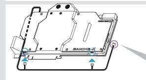
Once the water block is in place, plug in the remaining RGB LED cable connector to the water block as shown in the illustration.
