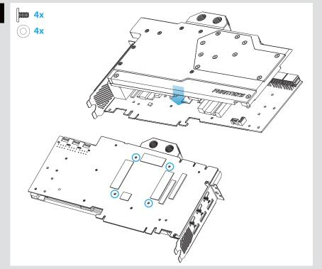
Make sure to lay the GPU with the water block flat down without resting on the PCI bracket.
