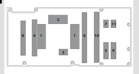
Make sure to remove the protective film on both sides of the thermal pads.
