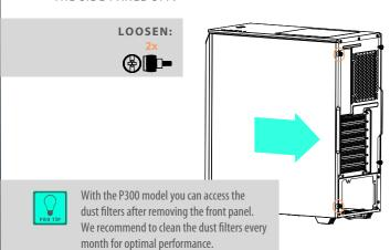
REMOVE FRONT PANEL BY PULLING ON IT FROM BELOW
