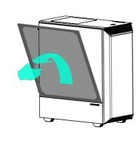
**C.** PULL UPWARD TO REMOVE.
