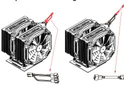
Plug the two fan cables to the Y-Splitter cable. Plug the single end of the fan splitter to the 3-pin end of the PWM adapter. Connect the PWM to the 4-pin on the motherboard.
